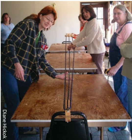
Twisting individual plies with a rope-maker's crank
