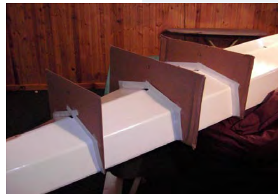
Making temporary external forms from the SOF hull
