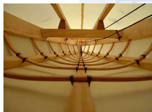
Figure 1 Pieces of dowel at the bow and stern provide a way to rig a pulley cord for float bags.
