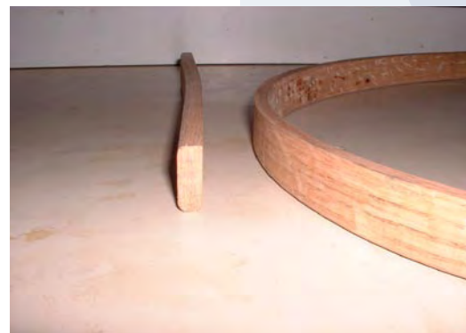
Figure 2 It is easier to round over the edges of coaming stock prior to bending it. Leave the lip edge square.
