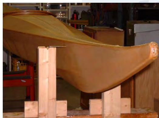
Figure 4 Supporting the kayak for finishing with nails temporarily inserted into drilled bow and stern loop holes in the gunwales.
