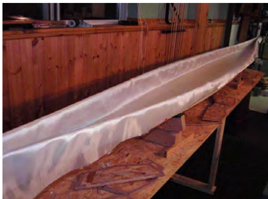
Western red cedar strips laminated with 4-ounce fiberglass resulted in a final weight of 30 pounds.
