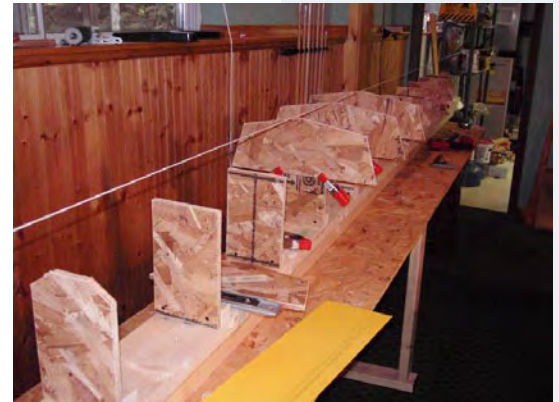
Attaching plywood forms to the strong-back, matching the rocker measurements recorded earlier
