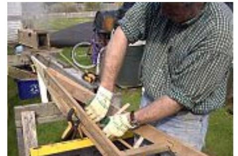
For pieces of wood I know to be difficult to bend I'll use an old rifle sling as a backing strip, an old leather belt would work as well.
