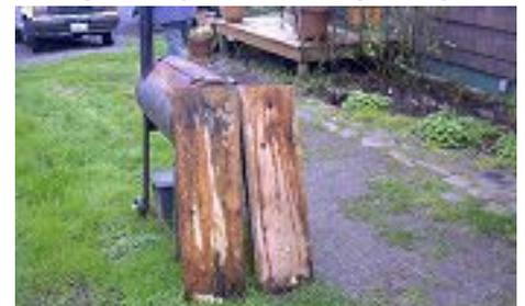
I built this box about 4 ft. long and about 6-inch square. I wanted something that I could steam four or five ribs at once. It needed less interior volume than the 8 ft. box I use for steaming coamings.
