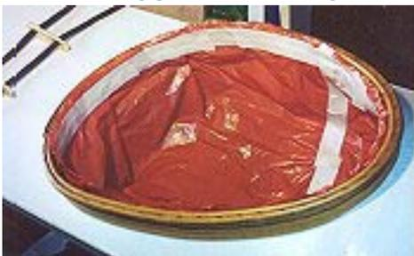
Before removing this plastic pattern from the kayak, it helps to add some additional tape to guide the transfer of the pattern to the fabric. Run a piece, centered under the foredeck from the cardboard toe piece to the front of the coaming. Also mark the center back of the coaming. Carefully remove the plastic from the boat.
