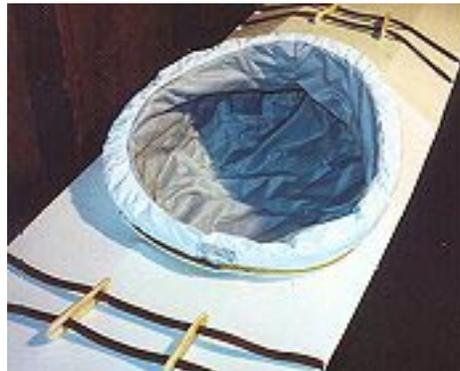
Be sure and practice recovery skills with the sock in place as the fabric can present some interference to slipping back into the cockpit. Also remember, the sea sock must only be used in combination with another source of floatation. As such, it is a valuable piece of kayaking gear, providing a second line of defense, as well as keeping grit and grime out of the boat.
