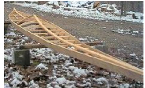
Following the *ayak* were the *masirosigik* (lighter, arched deck beams) of which there are two in front of the *masik* and ease the transition from the *masik* to the *ayak*. These were made from a 2"x6" purchased from Lowes.
