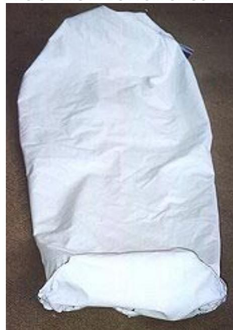
Determine the distance from the inside of the coaming, around the coaming rim, back into the base of the rim. Double this dimension and add 1½". Also, determine the circumference of the outer edge of the coaming rim and add 2". Cut a strip of fabric to these dimensions, piecing together a couple of sections if necessary. Fold in half lengthwise, coated side out, and sew a ¾" seam down the folded edge. This will form the bungee cord sleeve. Sew another seam 1" from the opposite edge.
