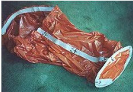
Before cutting this three dimensional pattern into a flat one, mark some match lines along every cut line. These are around the circumference of the toe section and along the center of the foredeck tape. Cut along both these lines, leaving the bottom of the toe section attached to the main body to avoid having a seam here.
