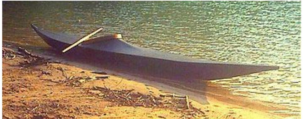
weathercocking into the wind. The cross section of the multi chine tends to be broadly rounded in the sukaut class and flat bottomed in the usiyut class. The narrower more rounded cross section of the sukaut class being safer in big seas as it was less likely to broach.
