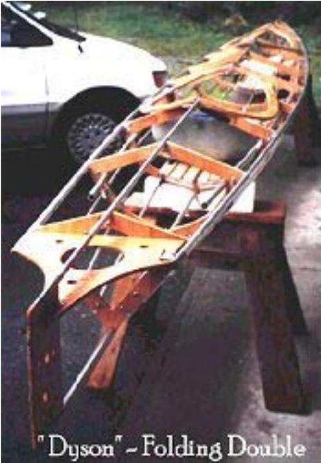
The first time I saw a commercially produced Feathercraft folder, I knew that the stringer to cross section problem was solved. By snapping the tubing onto the High Density Polyethylene (HDPE) cross-sections, Feathercraft had eliminated the need for mechanical connectors. For the homebuilder, it meant faster construction and assembly times, due to much less complexity. Also, since aluminum and HDPE require no shaping, sanding or finishing, additional construction time was saved.
