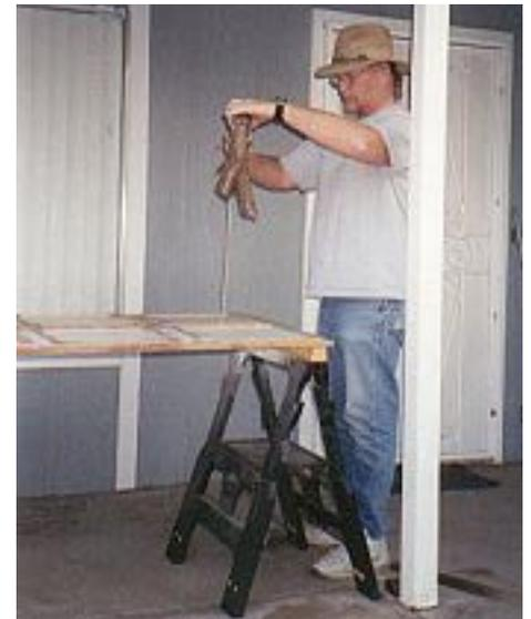
The branch started making marks in the nylon at 4', cut the finish at 6' and broke a couple of fibers and peeled up finish at 8'. Still, it was mostly sizable dents up to 10' and little real damage. It didn't break any fibers in the polyester skin but did make some serious dents and a couple of scratches.
