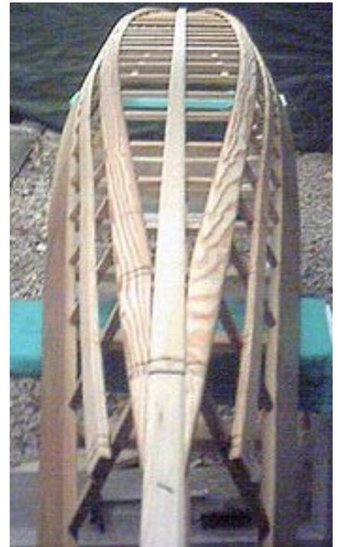
The *paliqviq* (cockpit coaming) is made of two separate pieces of red oak 2 1/2"x3/4". One being a U-shaped piece and the other is the flat back, pinned and glued together. Mine measures 28"x17".
