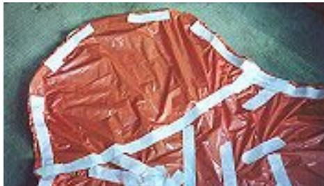
Fabric for the sea sock should be medium or lightweight coated nylon. If lightweight is used it may need reinforcement at heavy wear areas (at foot rest, under heels). These can be added later. The finished sock will have the coated side against the hull for the main body, but the coated side out for the coaming piece. This will improve the grip of the sock to the coaming and that of the spray skirt to the sock.
