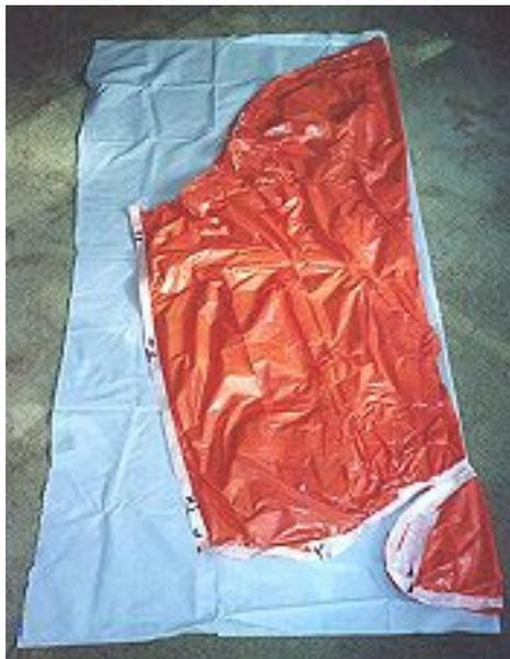
Draw around the pattern onto the fabric adding about 1½" to all dimensions. This provides some excess to prevent the fabric from being in tension if the sock shifts a bit in the cockpit. Mark all matchlines onto the fabric, then cut out all pieces.
